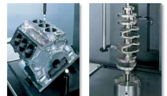
Measurement example of cylinder block and crankshaft.
