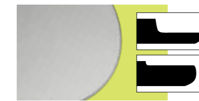
Terrace Grinding Counter Measure against Knife Edge/Asymmetric Profile Grinding
