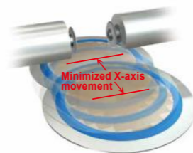
TWIN Dicing concept with the face-to-face twin-spindles
