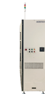
Energy sharing method-based charge/discharge testing system
